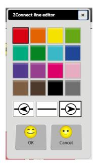
Select the line colour and the direction of the arrow accordingly. Links can be made in different colours so they are easy to see.
